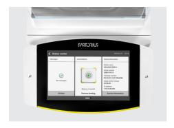
3. The Cubis® II Status Center shows all information about your balance and environmental conditions, e.g. calibration, leveling, temperature, humidity, air pressure and service, centralized in a dashboard. In case of warnings or errors, you get detailed help and support.
