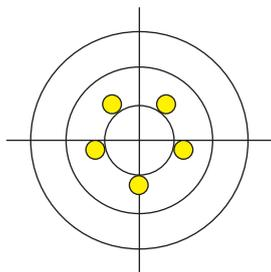
Result is precise, but not accurate: There is only minor variation between pipetting results; however, the mean volume differs from the set volume.
