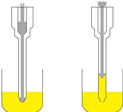
How a positive displacement pipette works
